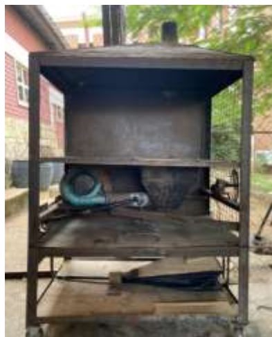
Figure 4: Developed mechanized open-hearth furnace
