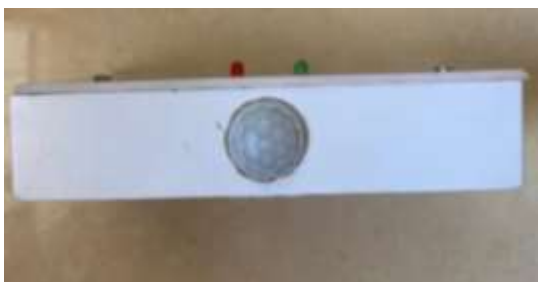
Figure 7: A View of the PIR sensor on the hardware device
