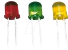
Figure 4: Light emitting diodes [24]
