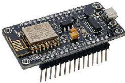
Figure 1: NodeMCU ESP8266 microcontroller [27]
