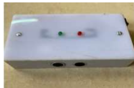
Figure 8: A view of the ultrasonic sensor on the hardware device
