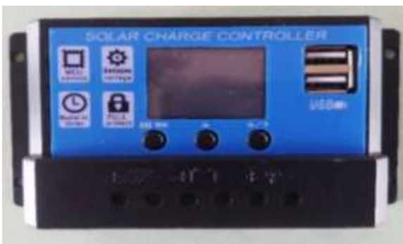
Figure 5: Solar charger controller
