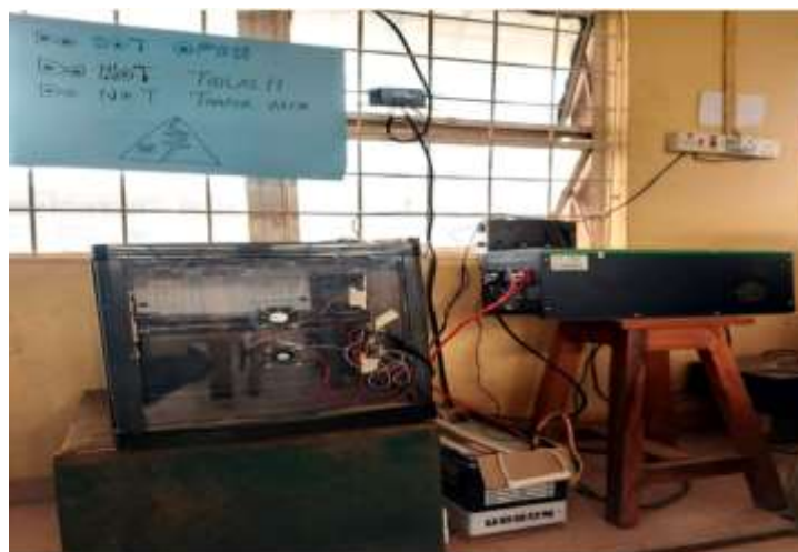
Figure 7: The developed hybrid instrumented onions storage facility
