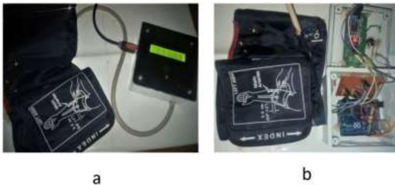
Figure 4a) Coupled ovulation detection device b.) Ovulation detection device under coupling
