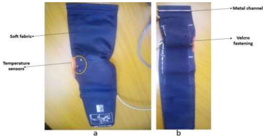
Figure 5 a.) Temperature sensors and fabric of the cuff b.) Parts used for holding the cuff in place
